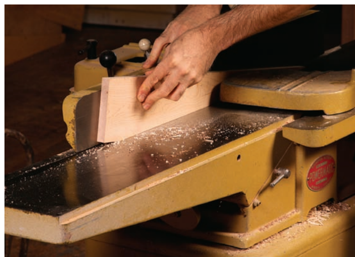
Joint the taper for a clean edge. It's fast and accurate. You also could use a handplane.
