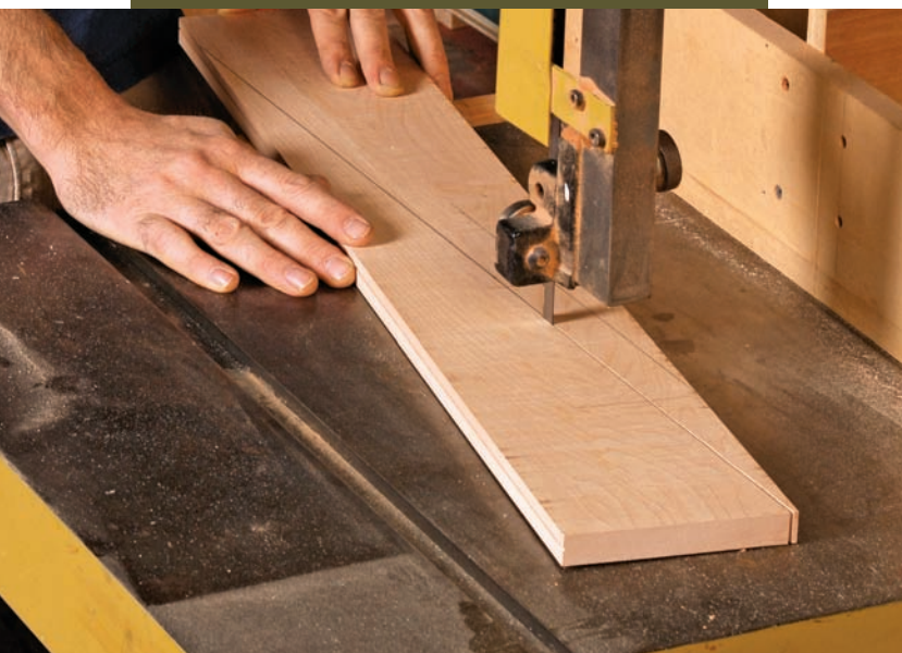
Taper the jig to match the tails. It should be several inches longer than the drawer sides.
