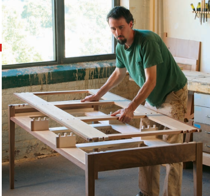
Drop the vertical dividers in place and top it off. With the vertical dividers glued into the lower stretchers, you can dry-fit the top stretcher assembly until the vertical dividers are set, and then glue the top assembly in place. Or use glue with a longer open time and do it all at once.
