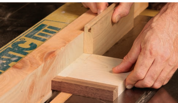
Graze the tenon cheeks. Before cutting the tenons, skim \frac{1}{16} in. of material from the tenon cheeks with a dado set. This gives a clean edge where the tenons end.
