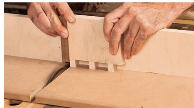
A simple sled. Hammer uses a very basic sled to hold the vertical dividers as he removes the waste between tenons. He works carefully to his layout lines without using a stop, test-fitting as he goes.
