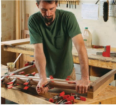
Glue in the spacers. Clamp the apron spacers into the leg-to-apron assembly.
