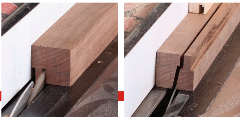
Rip tricks. The first two rip cuts form the tenon (left). Leaving the angled cheek cut for last lets the handle stock fall away from the blade (right).
