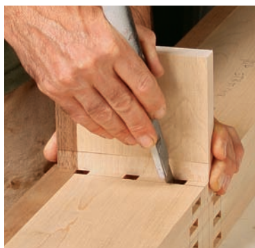
Mortises locate tenons. Use the mortises on the stretchers to locate and mark the tenons on the vertical dividers.
