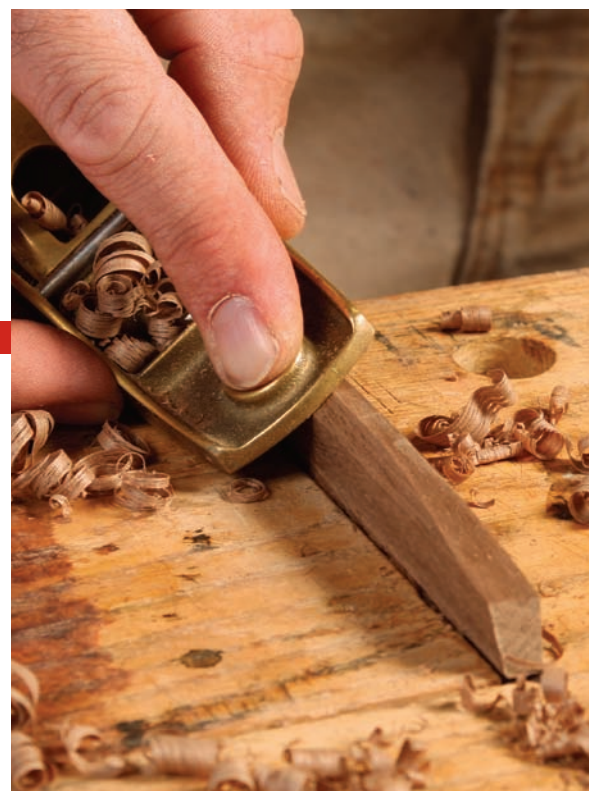
Final shape. Using the tenons to secure the handles in a vise, do the shaping with a block plane.
